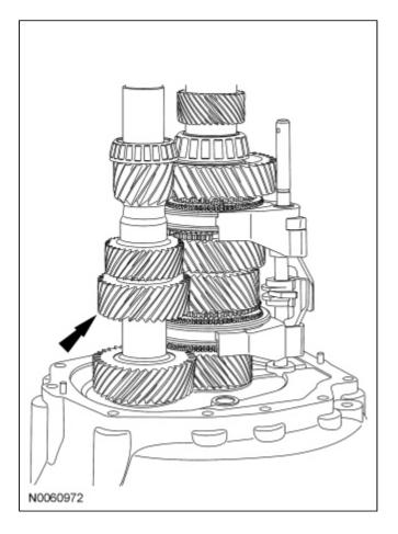
21. Install the 6th gear spacer and thrust washer.
